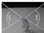
Measurement of flapping angle using high speed camera
